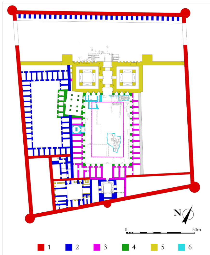
Figure 37. Plan of the palace showing the six main construction phases (elaboration by C. Passaro)
