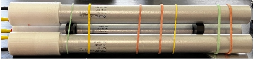
Fig. 2: The detector arrangement in our laboratory, which reproduces the original configuration used by Rossi. Our GMTs have a cathode diameter of 18 mm. On the right, a sketch of the arrangement in an orthogonal view.
