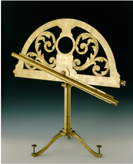
Fig. 2: Graphometer, Louis Chapotot, Paris, 1680ca, ©MPS, C III f 10.
